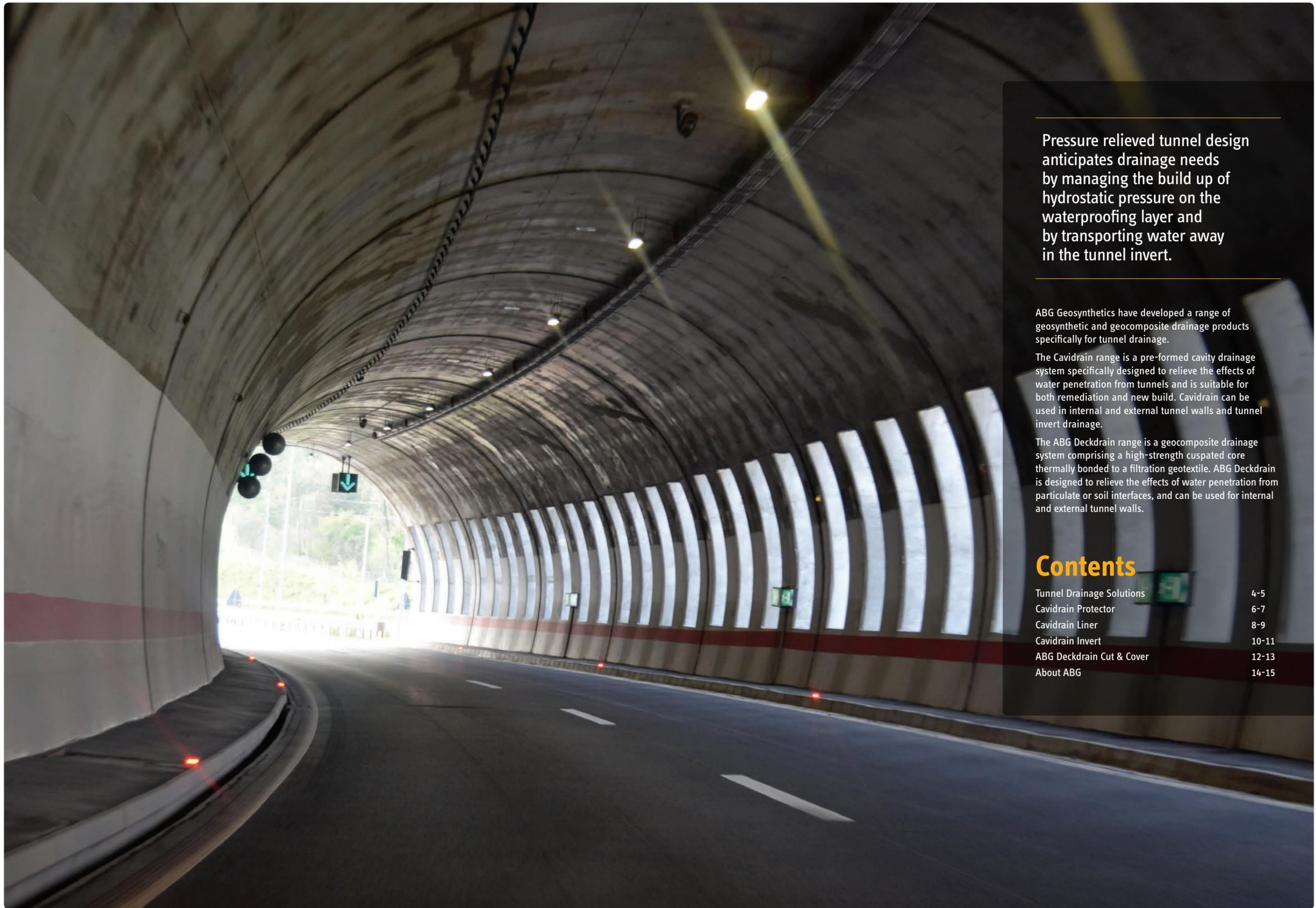
Pressure relieved tunnel design anticipates drainage needs by managing the build up of hydrostatic pressure on the waterproofing layer and by transporting water away in the tunnel invert.
