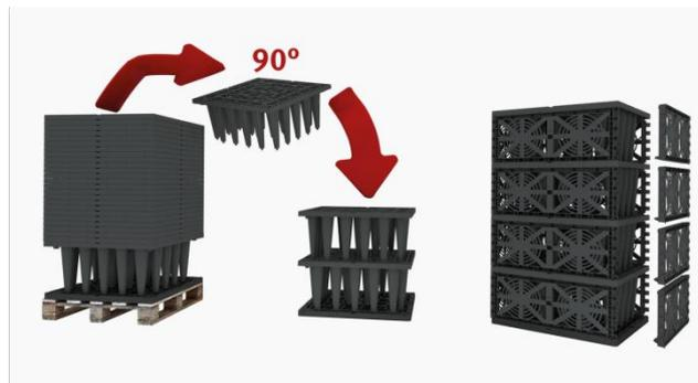
The stackable EcoBloc Maxx expands to 90% dry volume, optimising delivery volume resulting in one delivery to site. When stacked the available water volume gives 96% void giving a large storage volume in a small space. Side panels complete the tank.
