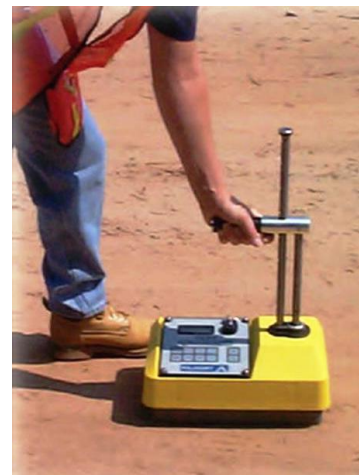
Figure 1: Nuclear density gauge
