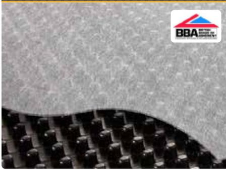
Deckdrain is a high-performance geocomposite drainage layer that directly replaces traditional granular drainage stone. When used in structural drainage, Deckdrain forms a robust drainage system designed to relieve external water pressure from buried structures such as behind retaining walls, on cut and cover tunnel construction, podium decks and roof gardens and buried tanks and service reservoirs.
