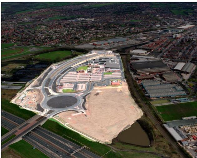
**Saturated arisings from M60 cutting stockpiled and used in highlighted area with Fildrain reducing consolidation time by 80%**
