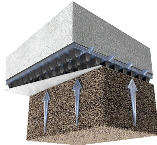
**Fig. 1: Deckdrain Reservoir Base Drainage cut-away diagram**
