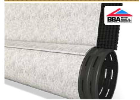
Fildrain drainage geocomposite is a cost effective alternative to traditional stone drainage. It collects and channels liquids and gases to a carrier pipe for transportation to a suitable discharge point. It has many applications in highway and embankment drainage.
