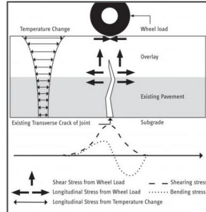
Fig. 1 - Mechanism of Reflective Cracking
