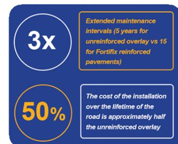
Fig. 7 - Extended asphalt overlay maintenance intervals & cost life savings
