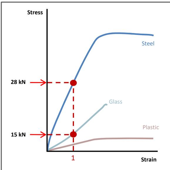
Fig. 2 - Stress strain curve of different reinforcement materials with similar cross sections
