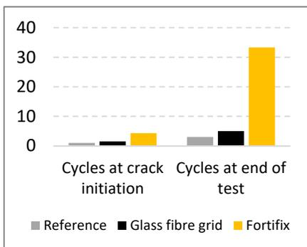
Fig. 6 - Maximum load and number of cycles to crack initiation and at the end of the test. Averaged results of the different anti-cracking systems expressed in number of cycles.
