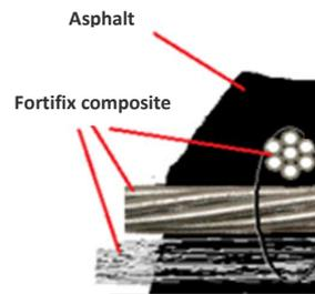
Fig. 5 - Fortifix steel-cord grid anchored into overlay to provide improved stiffness & bond
