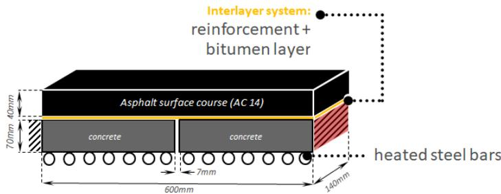
Fig. 4 - Thermal plate test setup with concrete/asphalt composite.
