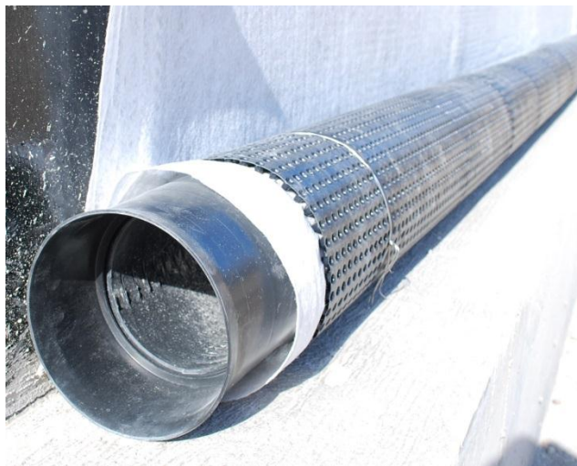
Deckdrain wrapped around perforated pipe feeding water directly into the pipe. Geotextile prevents backfill clogging inlet holes.
