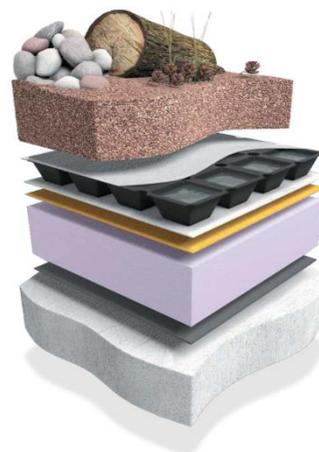
**ABG Green Biodiverse Roof System with carefully selected growing media and biodiverse features overlaying the ABG Roofdrain drainage composite**
